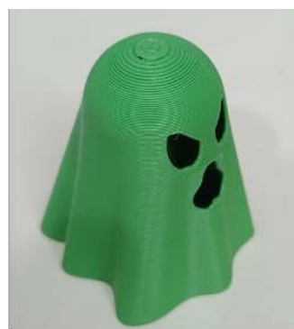
0.28 mm layer height print time: 28m 27s
