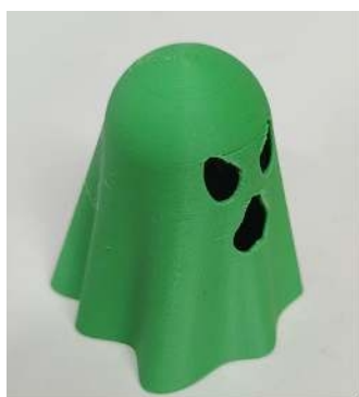
0.08 mm layer height print time: 1h 19m
