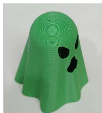
0.28 mm layer height print time: 28m 27s
