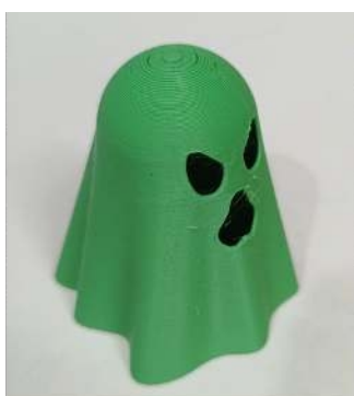
0.2 mm layer height print time: 36m 14s
