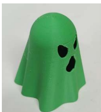
0.08 mm layer height print time: 1h 19m
