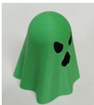
0.08 mm layer height print time: 1h 19m
