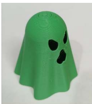
0.2 mm layer height print time: 36m 14s
